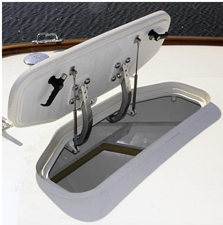
Hatch shown with 10-23-200 series Izerwaren Gas Springs. Picture: Freeman Marine Inc.
